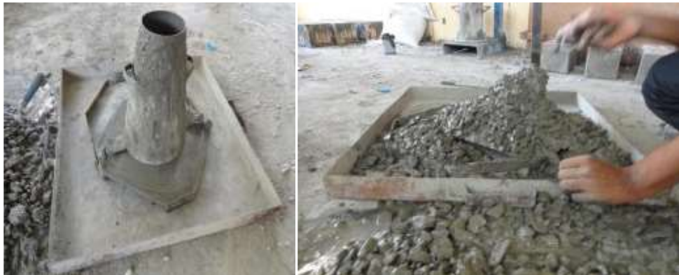
Fig: 2 Slump cone and collapse of concrete after lifting.
