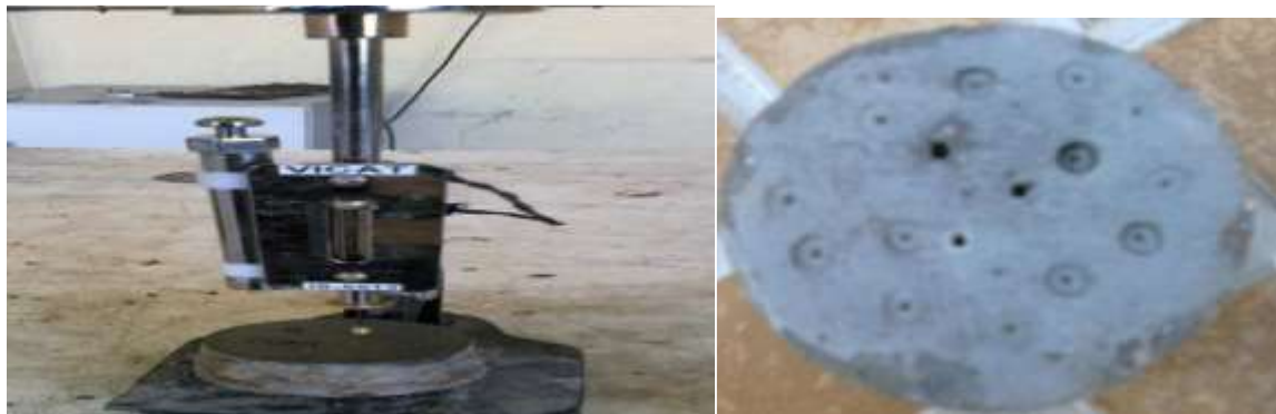
Fig.6 Test for setting time of cement
