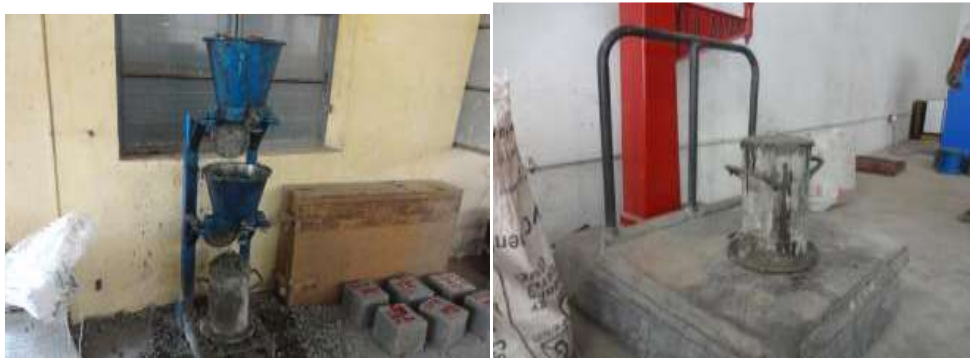
Fig:3 Compaction factor apparatus and weighing of partially weighed concrete
