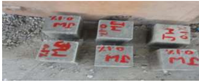
Fig: 4 Casted cube specimens.
