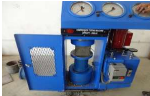
Fig: 5 Testing of cube specimen.
